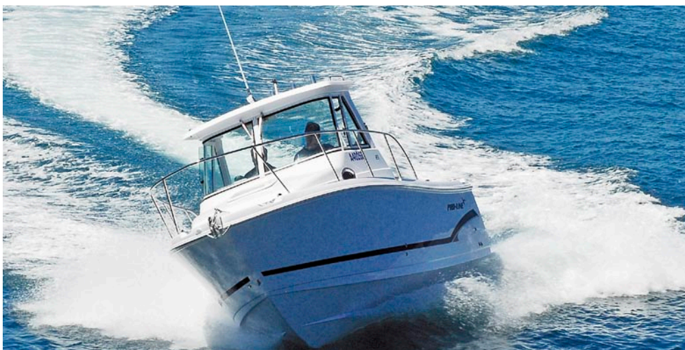
The twin 140 HP Suzuki's provided the 23 XP with a top speed of 38 knots at 6 300 rpm – quick for a hefty craft.
